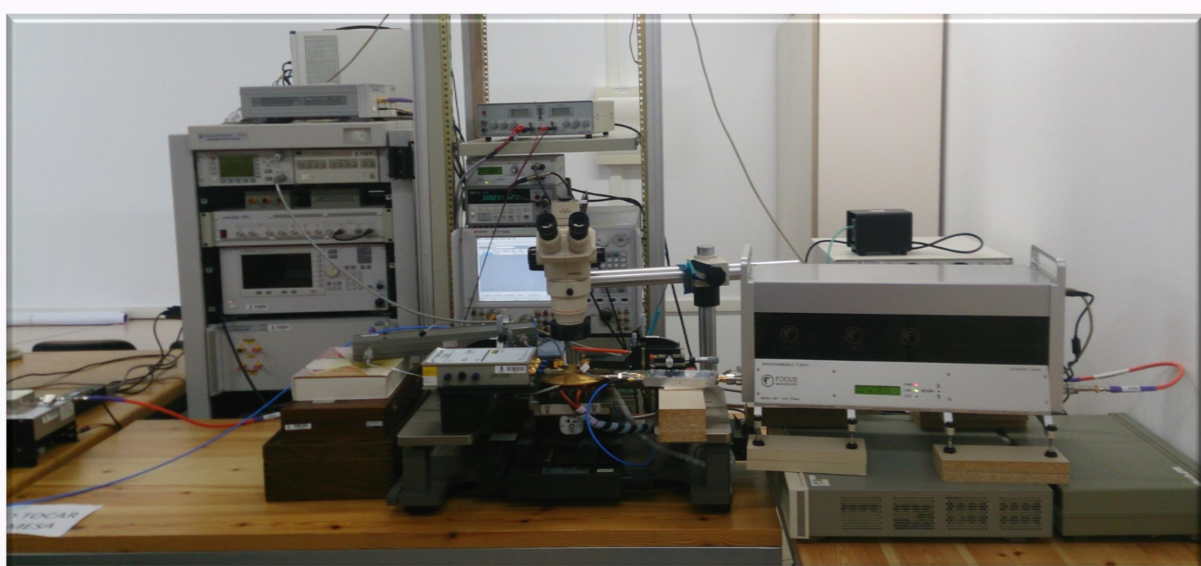
New meas. system PNA-X based set-up for 25W at Uvigo. Bandwidth: 2-18GHz.
