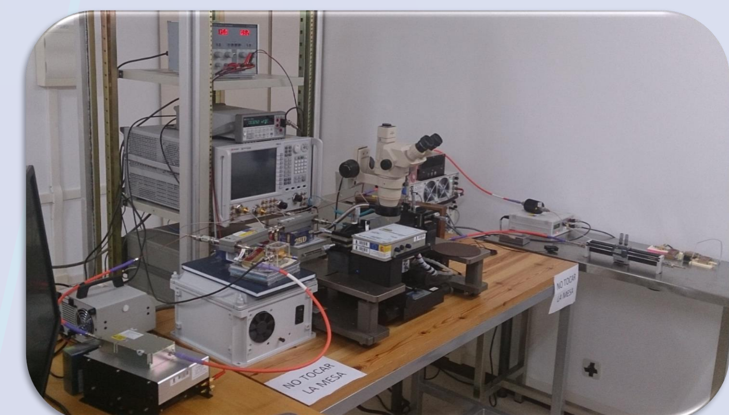
Meas. System PNA-X based set-up for 25W large-signal measurements at Uvigo
