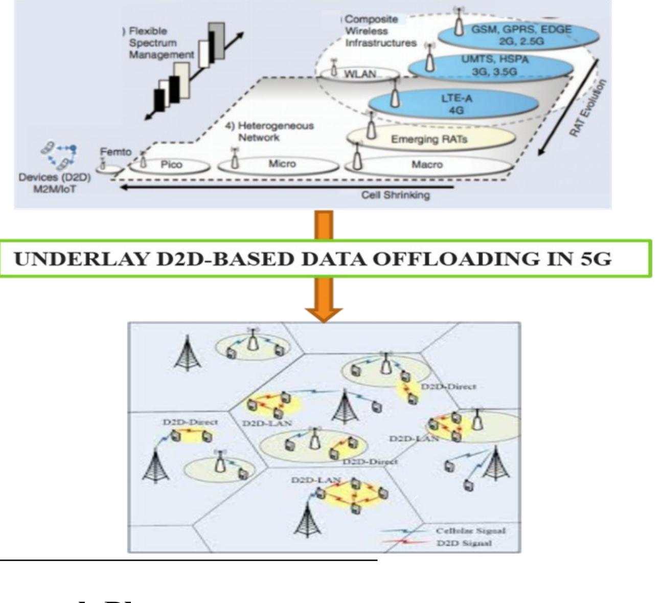
• Our main interest is underlay device to multi device (D2MD), here devices form a cluster/group with one device as head cluster for data offloading. This model inherit single transmitter to single receiver (unicast) challenges and poses more as: weakest receiver, head cluster selection, and users grouping. These points are poorly addressed in the literature compared to unicast cases and need more investigation [2,4].
