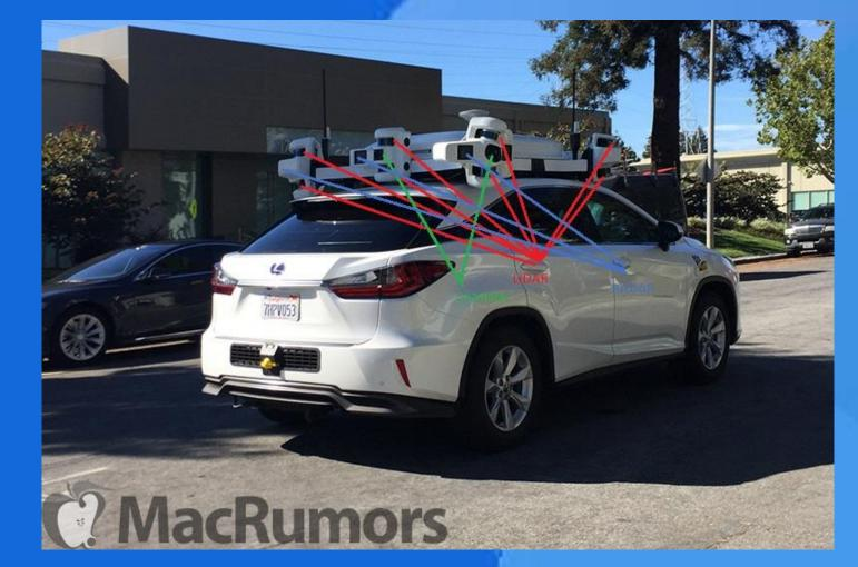
There are ADAS that can also use technologies not based in computer vision. For example, line keeping assistant system can rely in LIDAR or computer vision, or obstacle detection systems can be laser, radar, ultrasound or camera based. As mentioned in the motivation work, some technologies are more expensive than computer vision, but a comparative of the performance of the systems is necessary to adopt one or another.
