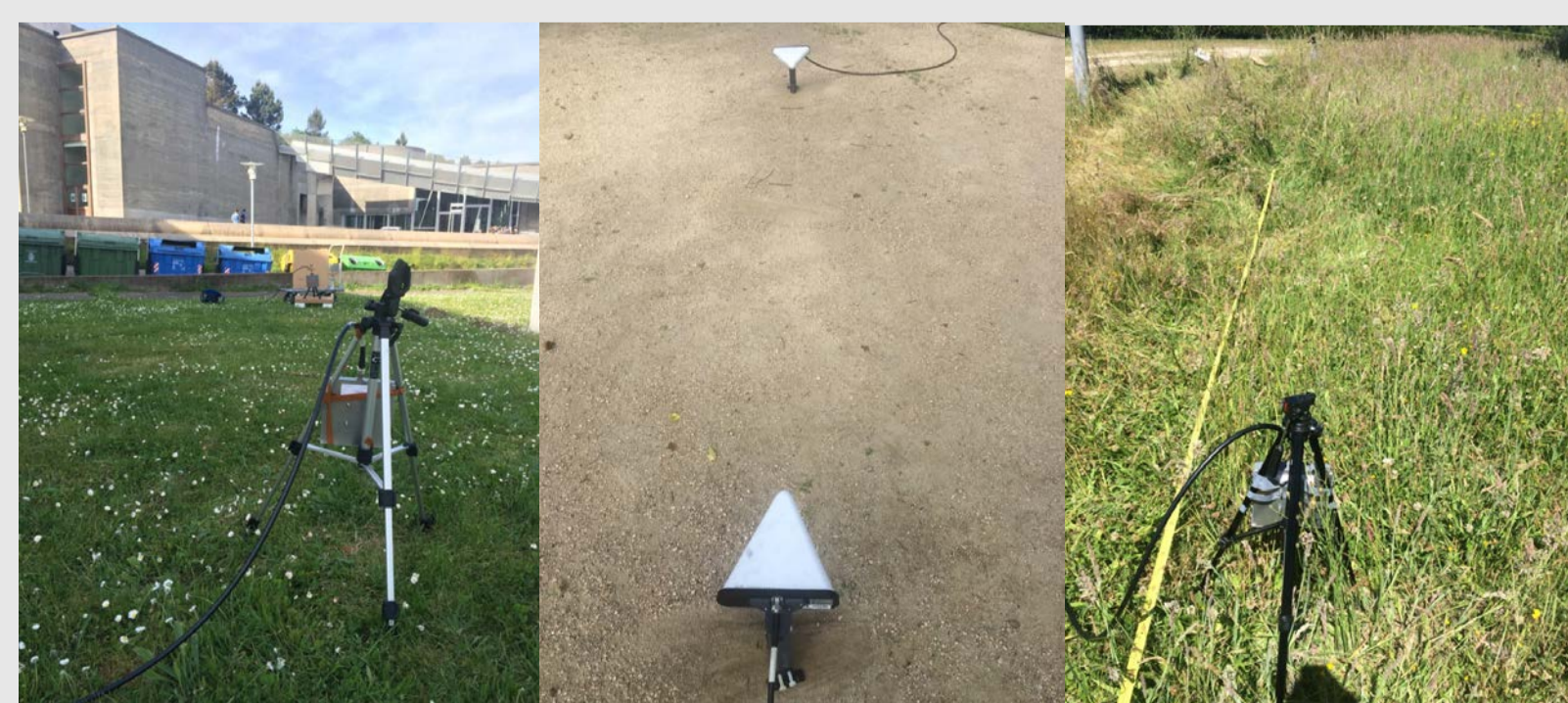
Fig 1. Path loss in agriculture fields at 2.4GHz for H1=20cm & H2=40cm.
